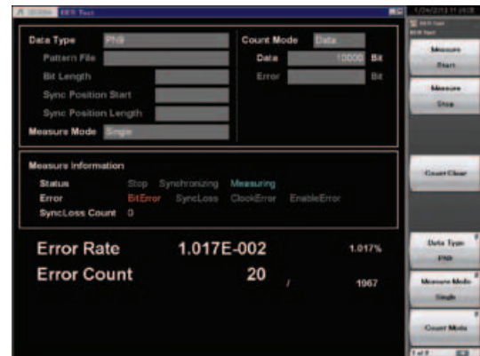
BER Measurement Function Main Screen
